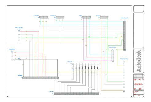
There are several drawing settings that can be made to suit this drawing style within the *Drawing Properties*. Wire numbers can be made inline and a gap between the wire number and wire defined:
