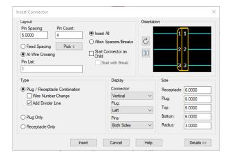
With additional functionality for editing, adding/deleting pins, reversing, splitting, stretching, moving pins, swapping pins etc and to define connector pin descriptions/usage.
